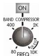
**STEREO:** In stereo mode, any of the ON switches will put both compressors in band compressor mode, however, the band compressor control will be independent in both channels, for that if you want that the band compressors work symmetrical, both controls will placed at the same position.
